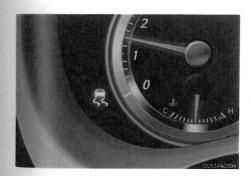
If the vehicle is in danger of slipping, or if the front wheels spin, the slip indicator light flashes to indicate that the VSC and TRAC systems have been engaged.
